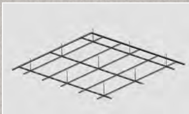
A / Grid installation (optional) Install Chicago Metallic™ Monolithic grid.
